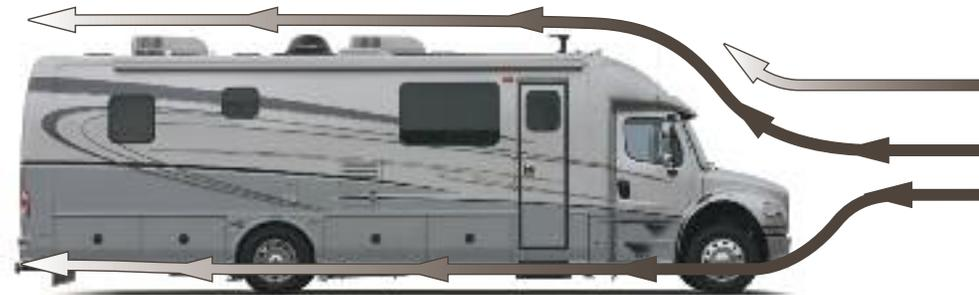
Body contours channel air flow up and around the motorhome cutting through wind, while increasing fuel economy and optimizing aerodynamics.
