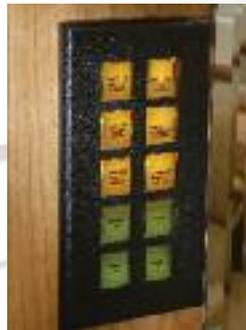
*The Intellitec Multiplex Lighting System with memory is accessible from four locations throughout the DynaQuest XL. This convenient system allows the user to completely shut down all of the 12-Volt lighting, from ceiling to floor, by holding one button down for a few seconds. Controls are located in the overhead console cab area, entry door, bathroom (near the vanity sink), and in the bedroom overhead cabinet.*
