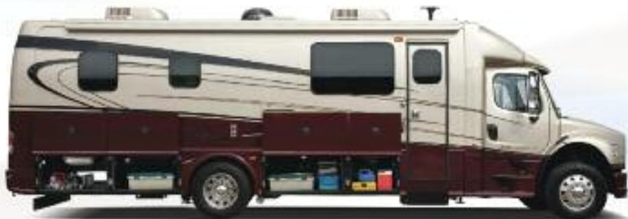
DynaQuest XL Model 340 has four large exterior storage compartments on the curb side of the coach with a rear pass through compartment. Powder coating inside and out, inhibits exterior storage compartment corrosion.
