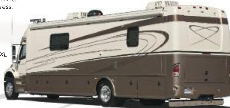
DynaQuest XL is standard equipped with LED tail lights, eight docking lights and a stainless steel stone guard on rear. (Ivory paint scheme)
