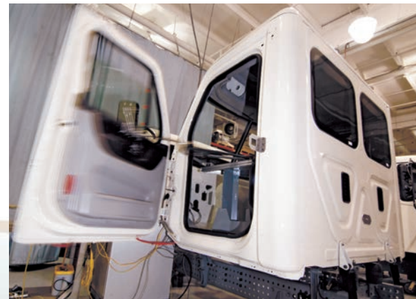
After 220,000 lock-unlock-open-and-slam cycles in engineering tests doors close just like new.
