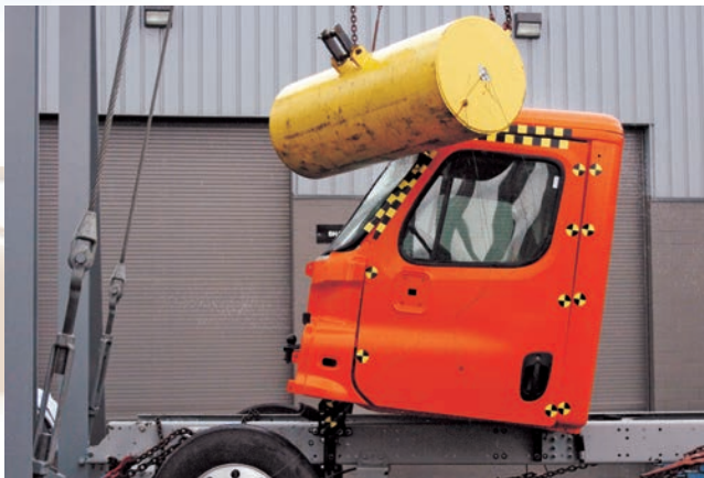
The cab design meets or exceeds stringent Swedish and European ECE R-29 crash test requirements for driver safety.
