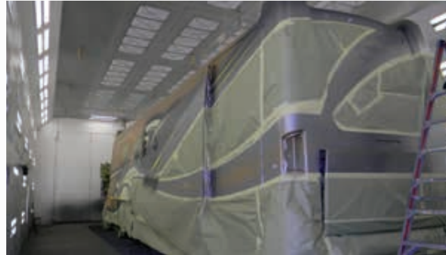
After masking to protect the previous coat, the unit is ready for black metallic base coat.
