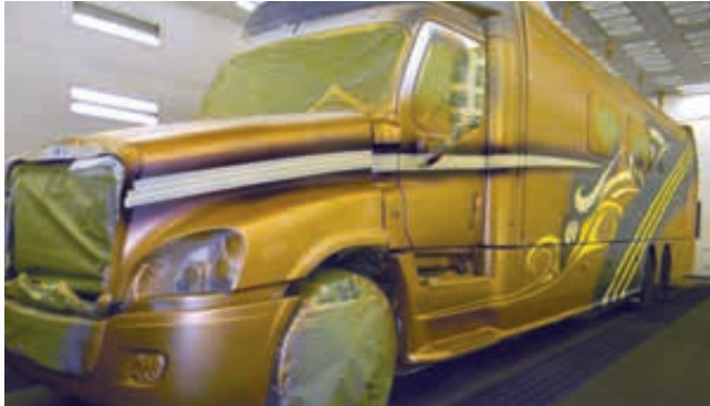
Digitally plotted, spray mask is carefully applied.
