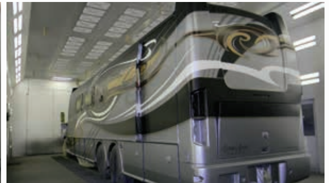
Final base coat color has been applied; the unit will be unmasked to prepare for clear coat.
