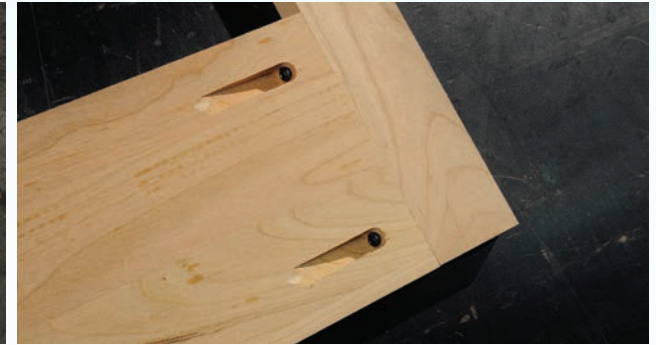
Pocket screws for structural integrity
