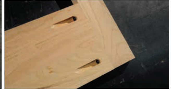
Pocket screws for structural integrity
