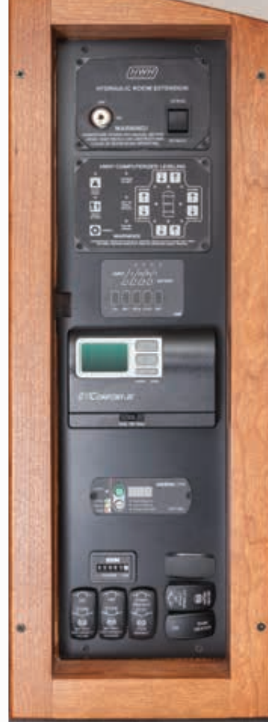
This panel, conveniently located behind the driver's seat, controls the living room slide-out, leveling system, monitor panel, heating/AC thermostat, power inverter, generator remote start switch and hour meter, water heater and heat pads for tanks.
