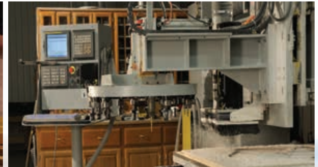
CNC routed custom Corian® countertops
