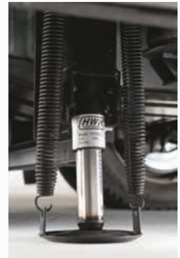
HWH CORPORATION The HWH fully automatic hydraulic four-point leveling system is standard on the F-Series.
