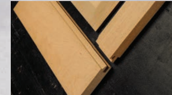
Mortise and tenon construction
