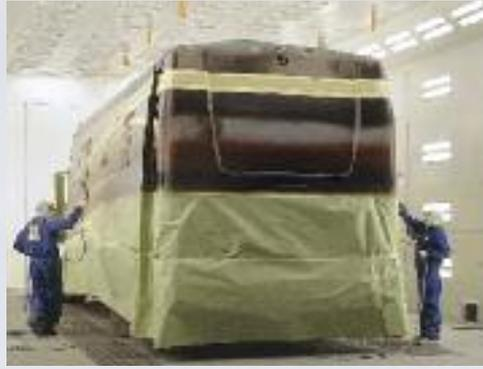
*Dynamax has three on-site 25' x 60' downdraft paint booths. This means we have maximum control of quality. By painting parts and slide-outs before they are installed, we eliminate overspray on slide seals and interior components.*
