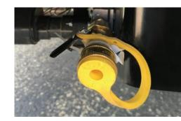
**LP Quick Connect** Each Isata comes with an LP quick connect for use with a portable grill.
