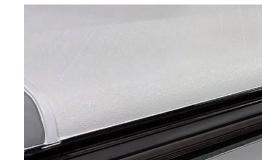
**Fiberglass Roof** This crowned, one-piece, fiberglass roof is more durable and easier to maintain than
